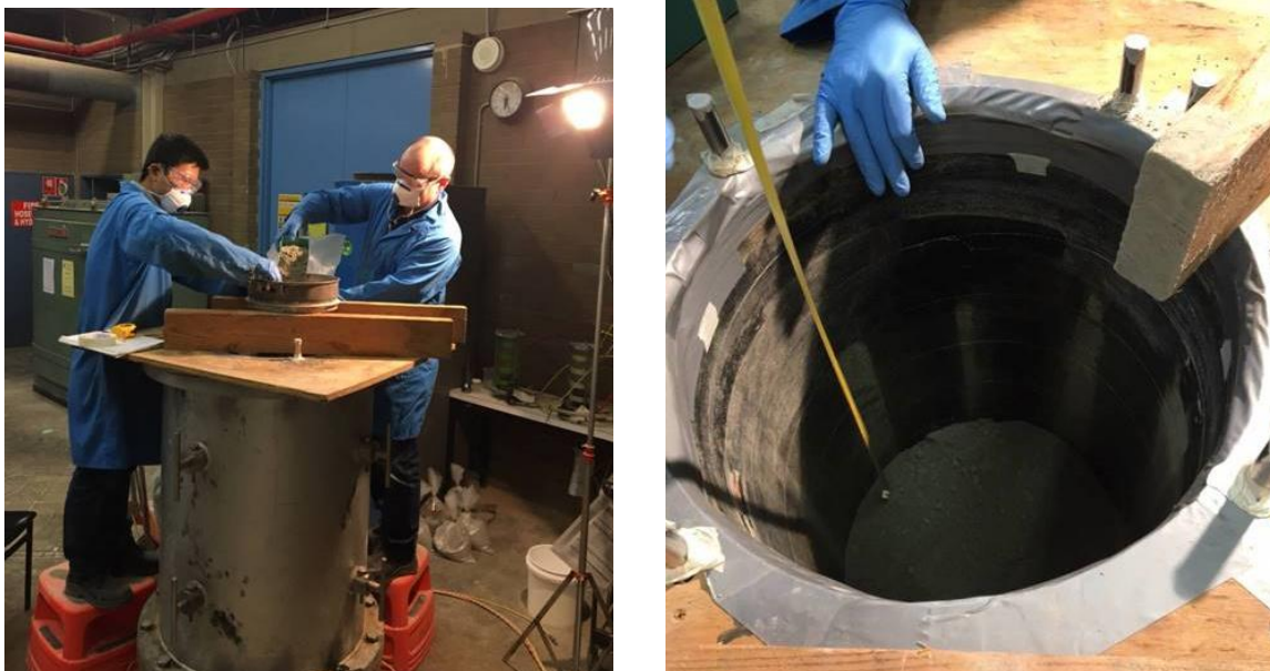
Figure 18. Dr Vo and Prof Russell prepare a tailings sample in the calibration chamber prior to conducting a CPT (left), and inside view of the chamber showing the sample being prepared (right).
